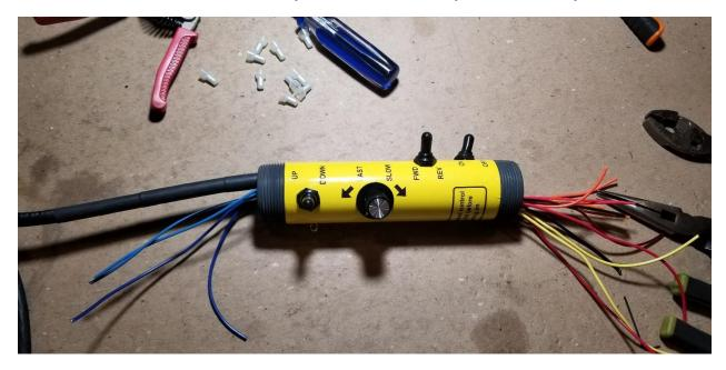
Next, cut each wire to equal lengths and strip them. Then twist the wires together and crimp them with the solderless connectors. Match each wire up. Blue with blue and blue/black with blue/black.
