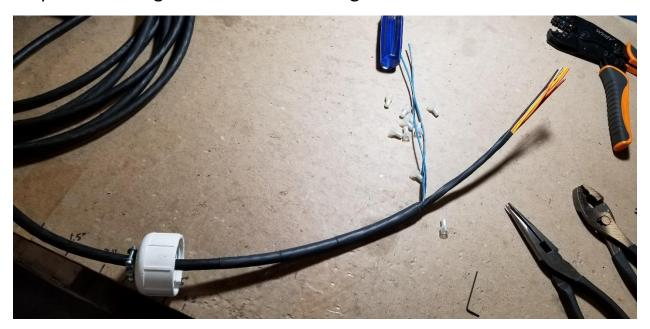
Then, insert the wire through the controller body, with the two blue wires bent backwards so they stick out the top of the body.
