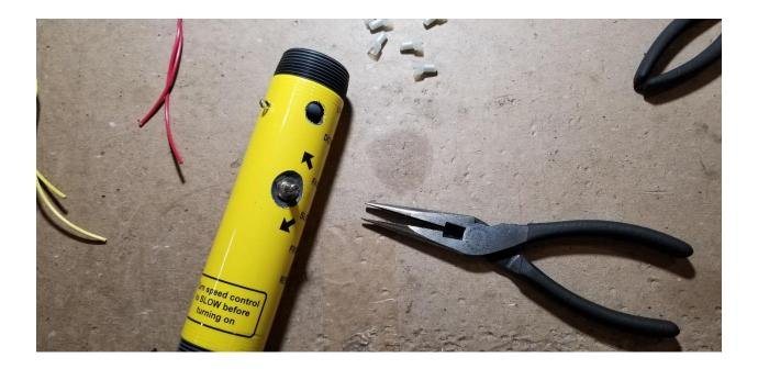
Next, insert the Up/Down switch. This is the switch with the blue, blue/black, and red/black wires. Insert with red/black wire protruding from the bottom of the controller and the blue and blue/black wires out the top. Secure with black switch boot. Using a pliers allows for a tighter fit.
