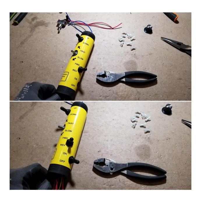
Next, use the hex key provided in the repair kit to secure the speed control knob. Elevate the knob just slightly so that it does not rub on the sticker.
