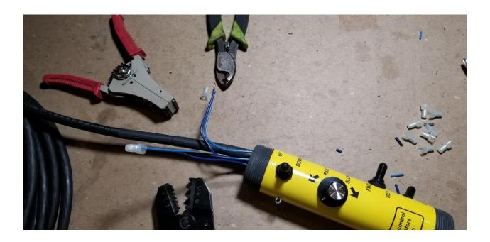
Tuck the wires inside the controller body and then twist the cap on tight. Before screwing the romex connectors down, make sure there is ample length to the wires out the bottom of the controller to work with.
