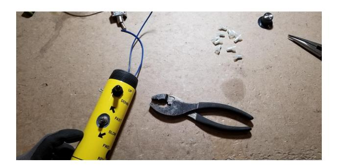
Next, repeat with the Forward/Reverse switch (yellow, yellow/black and black wires) and lastly the On/Off switch (red and red/black wires). Insert from the bottom with wires sticking out the bottom of the controller.
